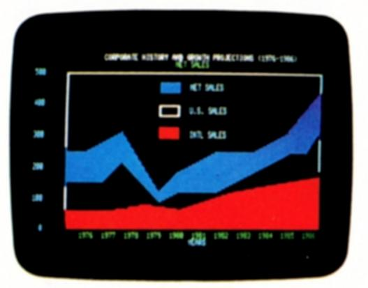
160 x 100 matrix of high resolution graphics. Dot or line drawing, powerful control directly from the keyboard. Eight bright, vivid colors include black, red, yellow, blue, green, magenta, cyan, and white. Monochromatic monitor provides three brightness levels for image highlighting.
