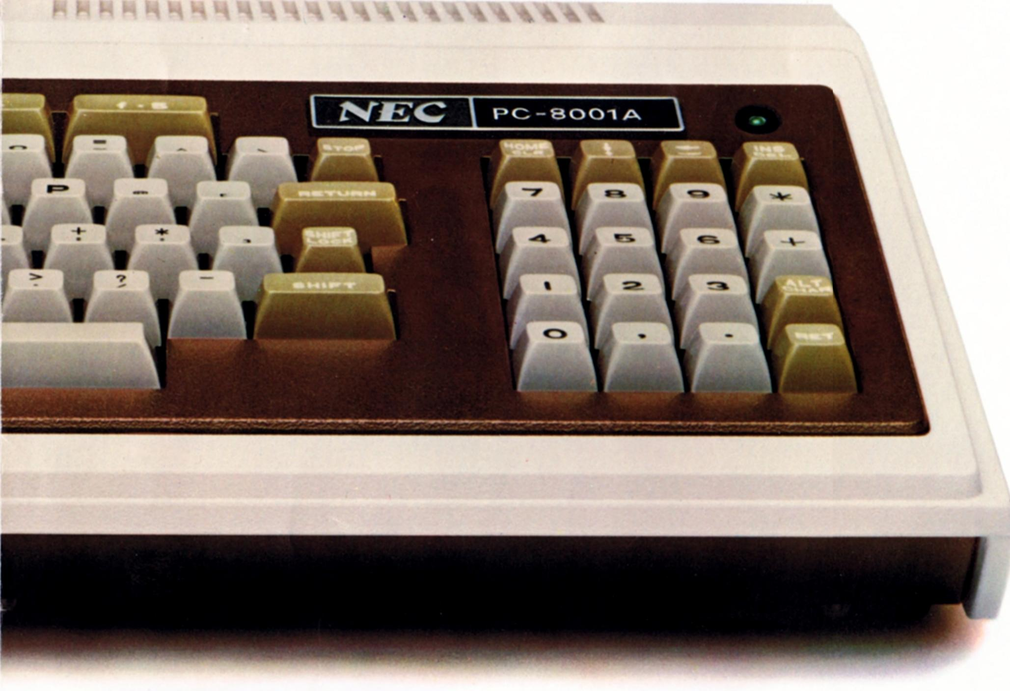
5 user-programmable function keys. (Our exclusive "no-panic" buttons. Up to 10 different user-defined routines can be activated using these keys and the shift key.)
