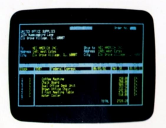
Screen formats of 20 or 25 lines and 36, 40, 72, or 80 characters per line, with adjustable scrolling window. A powerful editor simplifies programming and includes 4-way cursor control, character insert and delete, and much more, right from the keyboard. Terminal mode available with a single command.
