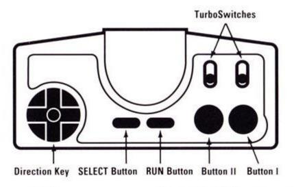
**Direction Key** (4-way controller) Press to move your paddle left, right, up and down
